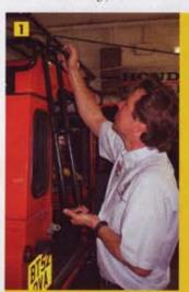
1 TJ removes the Defender's rear ladder before moving round to the front of the vehicle to disconnect the roof rack lights. 2 Meanwhile, Chris Simons works
